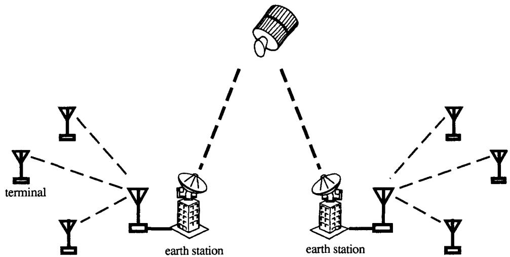
(a) terrestrial packet radio network and satellite packet network.
