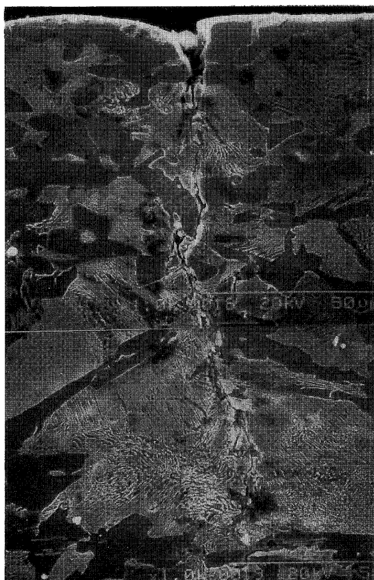
Fig. 7 Branching of cracks along microstructure of S45C specimens on cross sectional area in 561 K, 8 ppm
