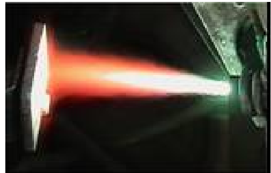
Fig.3 Appearance of feedstock material injected Ar plasma jet in the case of non-cooled nozzle use.
