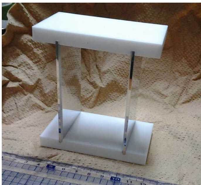
Fig. 4-33 Bending electrodes for muon beam deflection.
