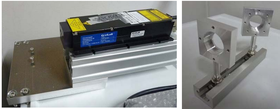
Fig. 4-8 Overview of LASER oscillator (left) and optical equipment (right).
