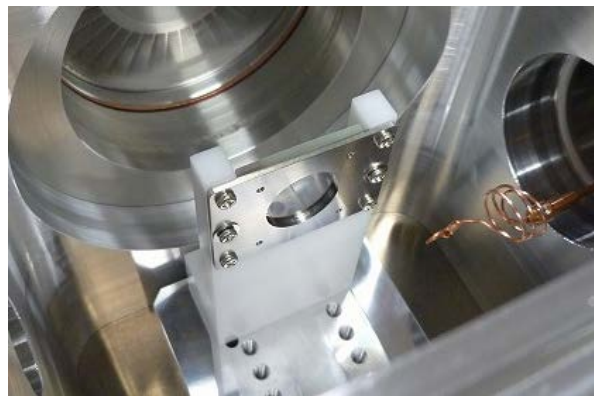
Fig. 4-7 Overview of micro channel plate (MCP) and holder
