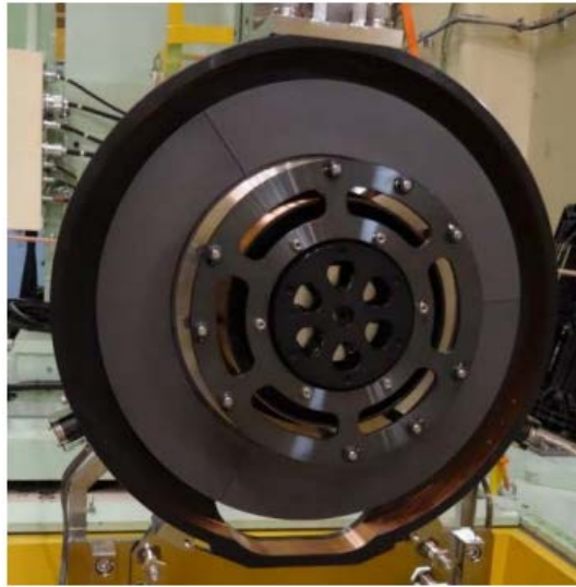
Fig. 2-3 Rotating muon target in the MUSE facility; installed in 2015 [43].
