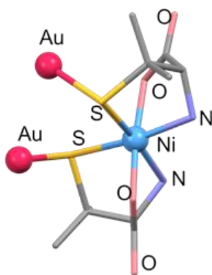
Figure 3-41. (a) Bis(tridentate- N,O,S ) coordination mode of the metalloligand, (b) coordination geometry of Ni II atom in [10].
