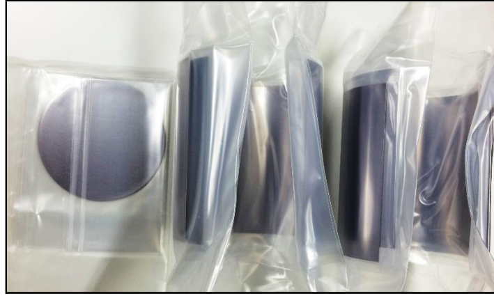
Figure 2.14: Vacuum packing of tantalum sample after acid cleaning procedure
