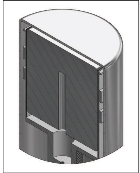
Figure 2.5: Inner configuration of standard electrode coaxial Ge detector produced by CANBERRA Industries Inc. [26]
