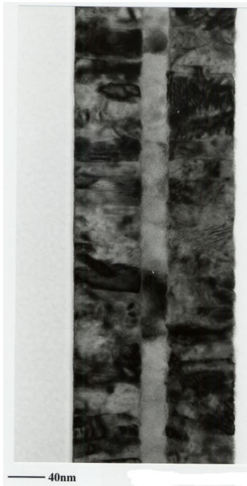
図 a-3-6 (b) 3層試料 (Mo(70 nm)/GSTB(30 nm)/Mo(70 nm)) の TEM 断面観察
