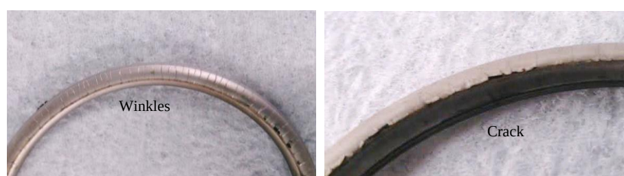
Fig. 5.27 Photos of o-rings after Ni plating. Winkles and cracks are induced owing to elastic strain.
