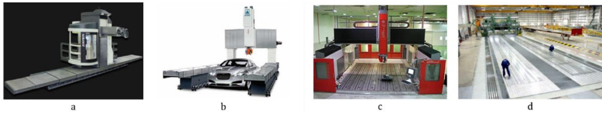
Fig. 1-3 Machine tools for large parts [1], (a) movable column, (b) gantry, (c) elevated gantry, and (d) large wing skin machining on a dual spindle gantry.
