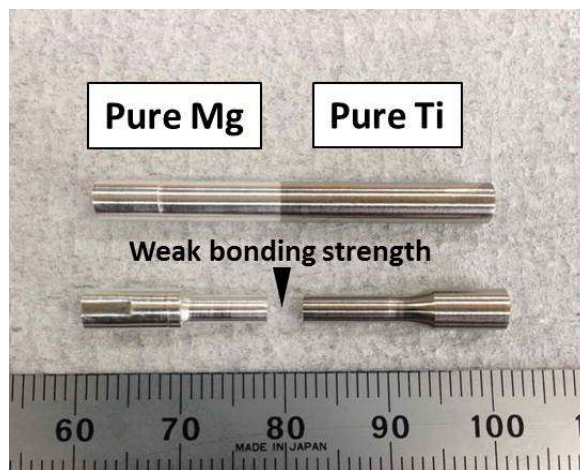
Fig. 4.16 Failure of pure Ti/pure Mg bonded specimen during machining.
