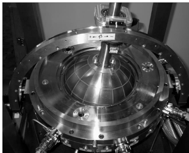
Fig. 1.10 3-DoF spherical synchronous actuator (Aachen institute of technology)
