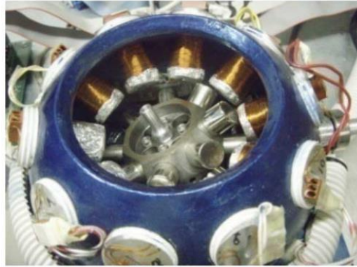
Fig. 1.11 3-DoF spherical synchronous actuator (Georgia institute of technology)
