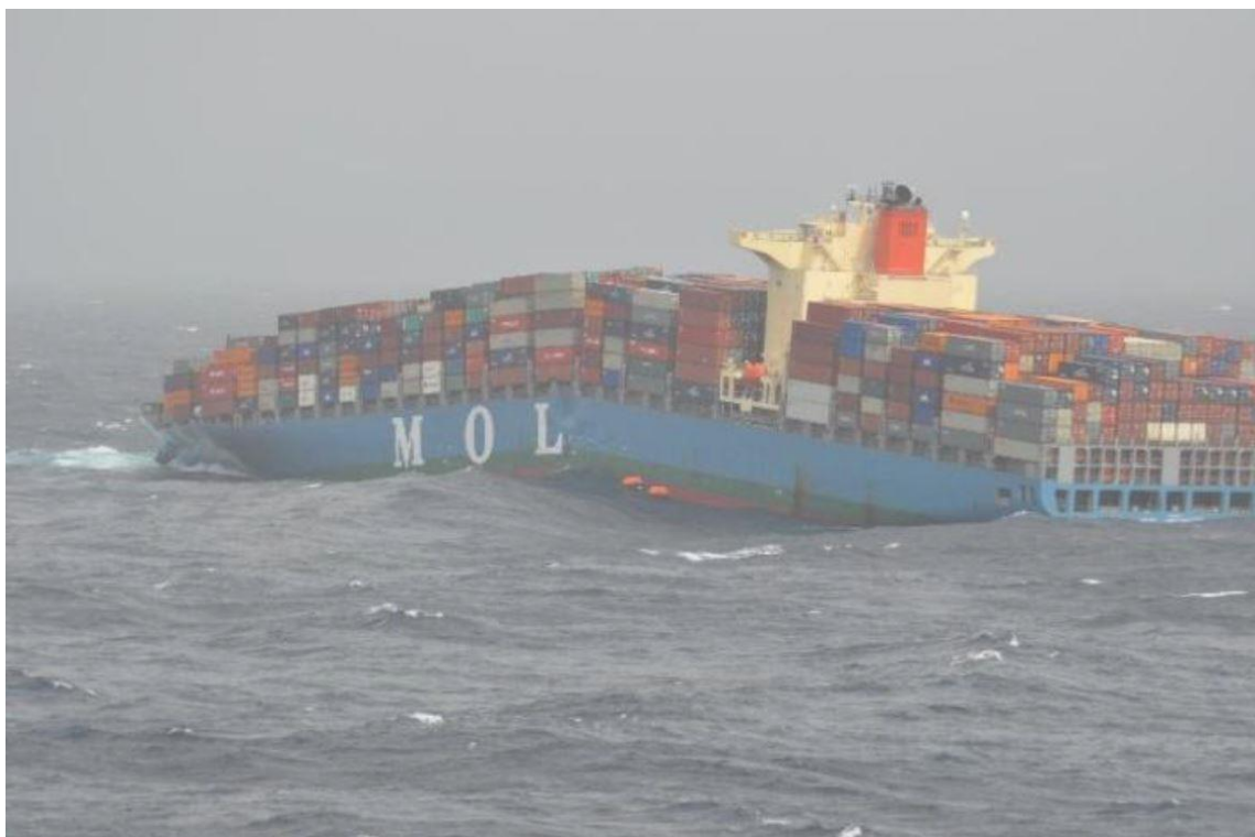
Fig. 1-2 Structural failure of MOL COMFORT[9]
