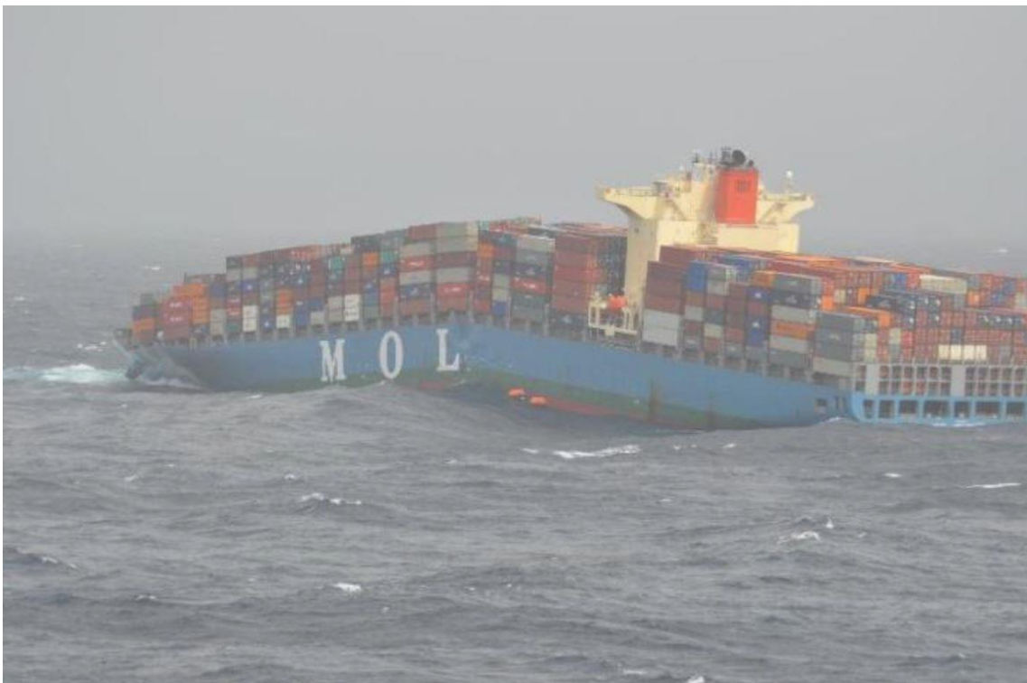
Fig. 1-2 Structural failure of MOL COMFORT[9]
