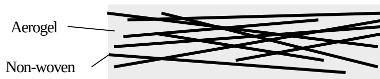
Fig.1.2 Overview of aerogel non-woven thermal insulator
