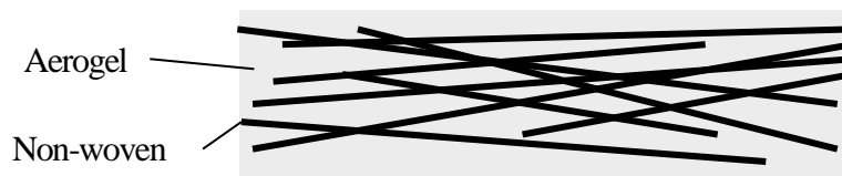
Fig.1.2 Overview of aerogel non-woven thermal insulator
