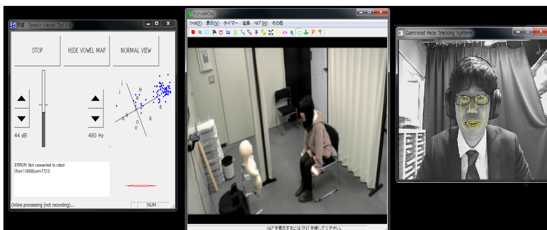
Fig. 3.4 Screenshot of operator interface (left: lip motion generation system, center: view of experimental room, right: head motion recognition system)
