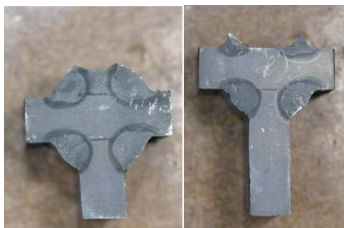
Existing wire(at weld toe and root)
