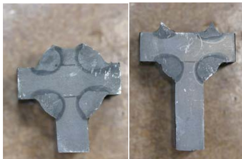
Existing wire(at weld toe and root)
