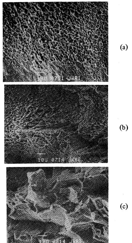
**Fig. 5** Fractographic investigations of center of fractured surface of tensile tested specimen of EBW joint
