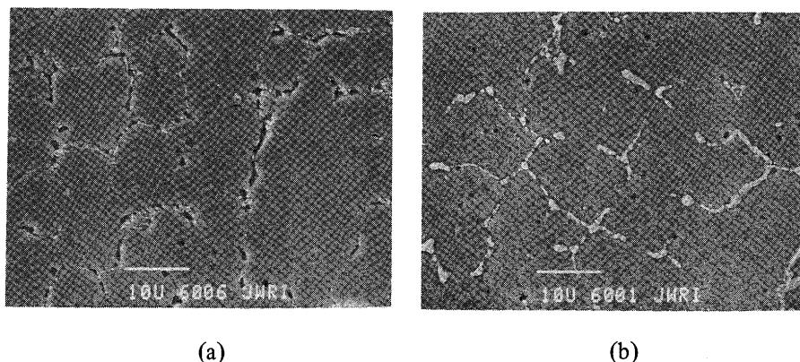
**Fig. 3** Typical microstructure in weld metal with SEM ( $\times 2000$ )
