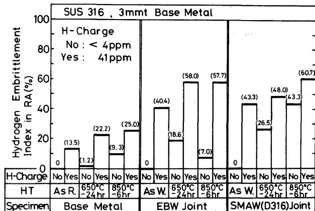
**Fig. 4** Effects of heat treatments and hydrogen charge on hydrogen embrittlement index in the reduction in area of the tensile tested specimen for base metal and EBW and SMAW joints
