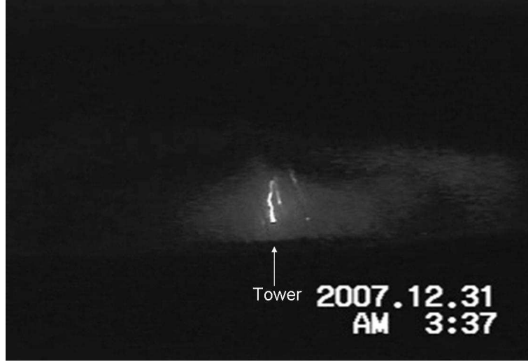
Figure 3.3: One image of the video camera installed at Site C for the upward lightning. The left luminous channel is the upward lightning, while the other luminous channel is the lightning flash occurred nearby.
