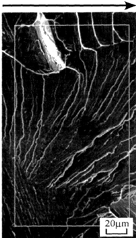
Fig. 11 SEM micrograph of fracture surface of type 444 ferritic stainless steel from Charpy impact test at 77K (standard image).
