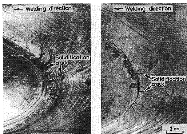
Fig. 10 Typical macrostructures in weld surface after the Trans-Varestraint test (a) DP-70HN (0.11%N, \delta : 77%) (b) DP-100LN1 (0.02%N, \delta : 100%)
