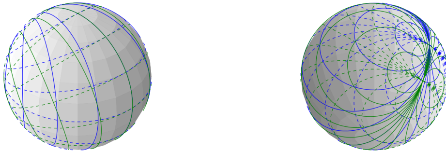
Figure B.1.2: Illustrations of the mismatch of the polarization bases. The direction of the basis for each polarization is shown as the line on the sphere. The left figure shows the front view, and the right figure shows the rear view. The solid lines represent the direction of the basis for the co-polarization, and the broken lines represent the direction of the basis for the cross-polarization. The blue lines are the definition with respect to the axis of the paraboloid, and the green lines are that with respect to the axis of the receiver. Here, the offset between the axes is 30^\circ .
