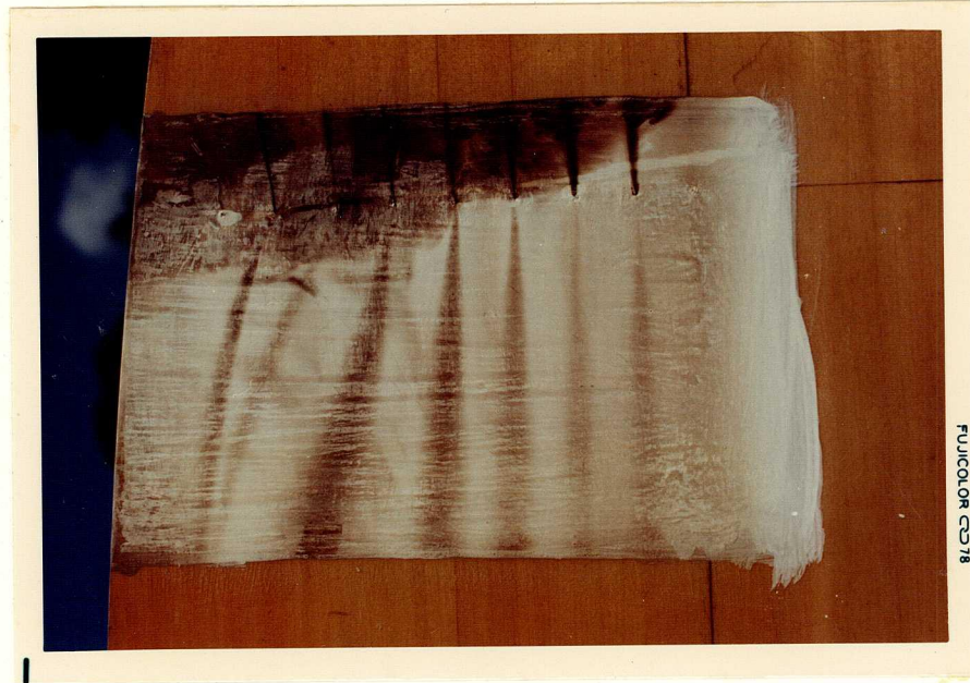
Fig. 1.45 (b) Limiting streamlines on bottom at S.S. 7.
