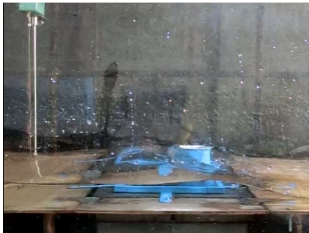
Fig. 5.15 7.5cm diameter tank with 100% oil drift and stops at the dike
