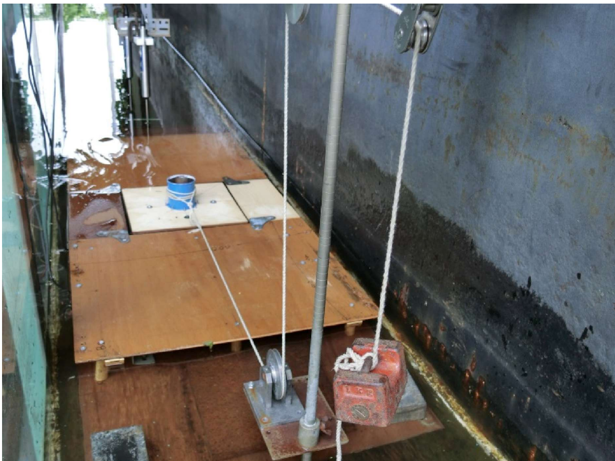
Fig. 5.9 Calibration of underwater load cell (load cell is attached below the tank)
