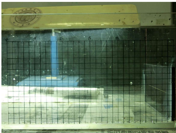
Fig. 3.2 The tank wall just before the oil reservoir was scaled finely with centimeter mesh
