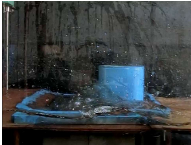
Fig. 5.18 16.5cm diameter tank with 50% oil drift and stops before reaching the dike
