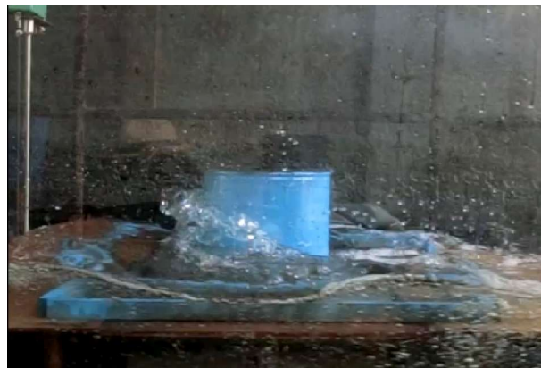
Fig. 5.19 16.5cm diameter tank with 100% oil remains stable in the wave
