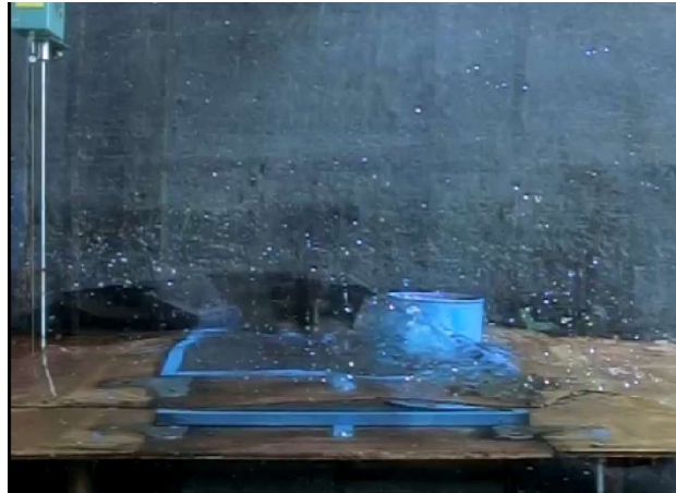
Fig. 5.17 10cm diameter tank with 100% oil drift and stops at the dike
