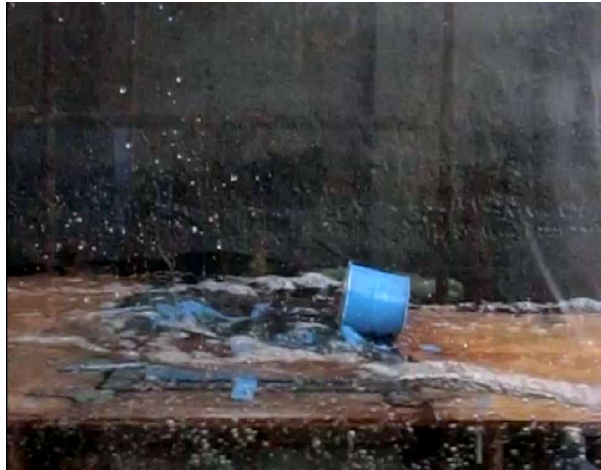
Fig. 5.14 7.5cm diameter tank with 50% oil tumbles by the dike before drifting
