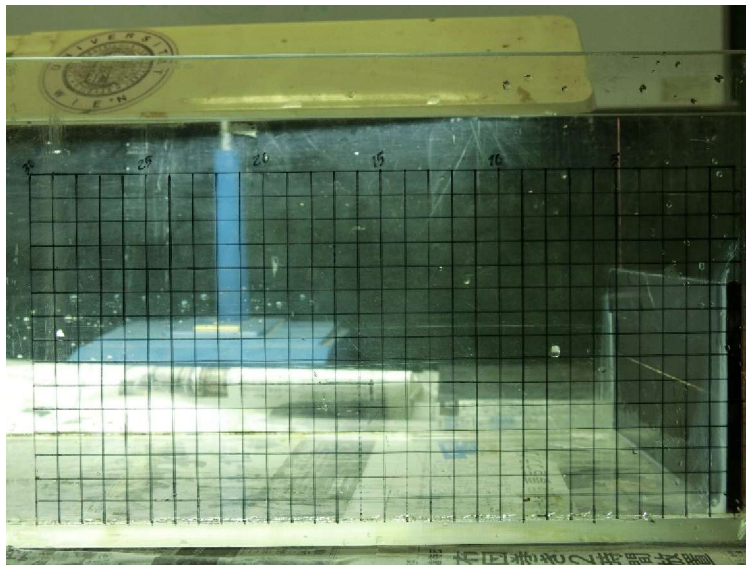
Fig. 3.2 The tank wall just before the oil reservoir was scaled finely with centimeter mesh
