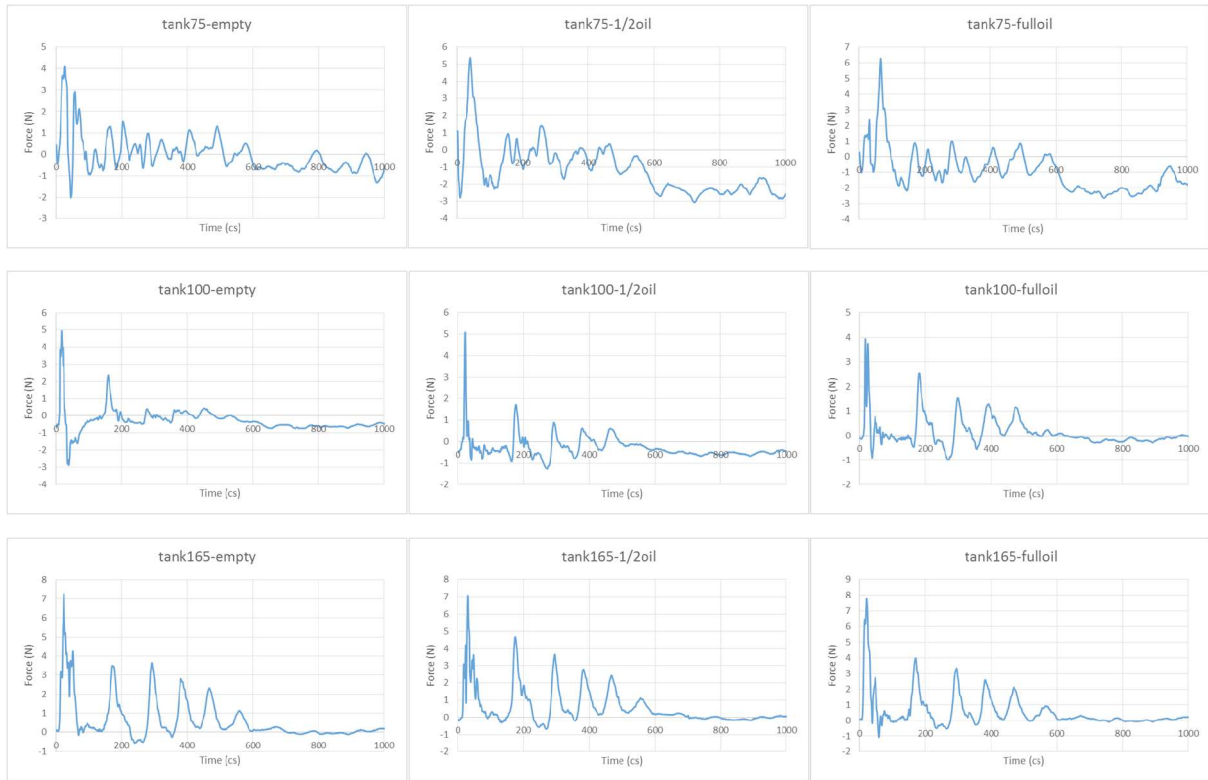
Fig. 5.12 Measured horizontal wave force on each tank
