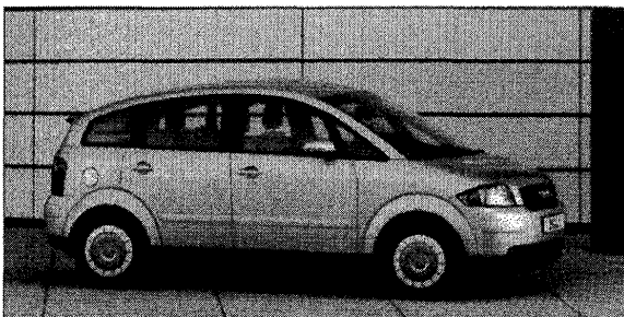
Fig.5 Audi A2 completely in Al.
