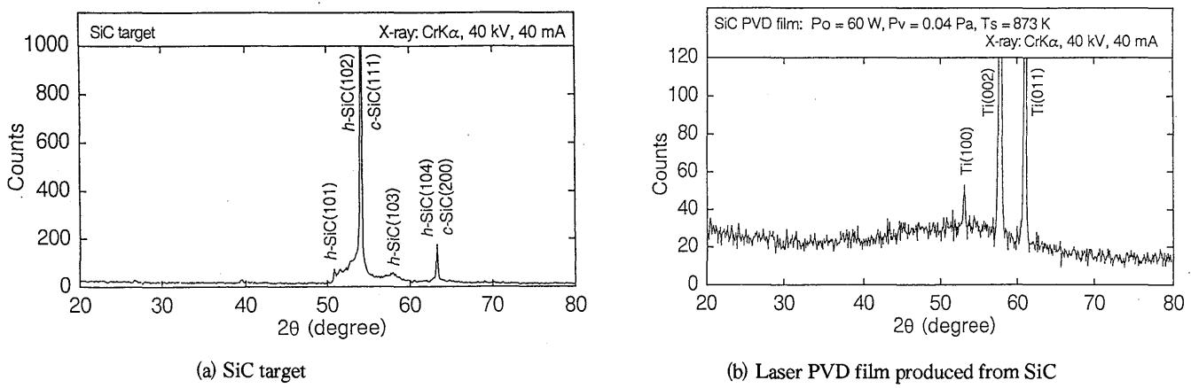
Fig. 6 X-ray diffractometer result of SiC target (a) and LPVD film produced on Ti substrate (b).
