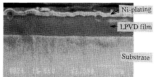
Fig. 3 SEM photos of surface and cross section of LPVD film produced from  $\text{SiC}$  target at  $P_v=0.03 \text{ Pa}$ ,  $T_s=723 \text{ K}$ ,  $f_d=0 \text{ mm}$  and  $DST=40 \text{ mm}$ .
