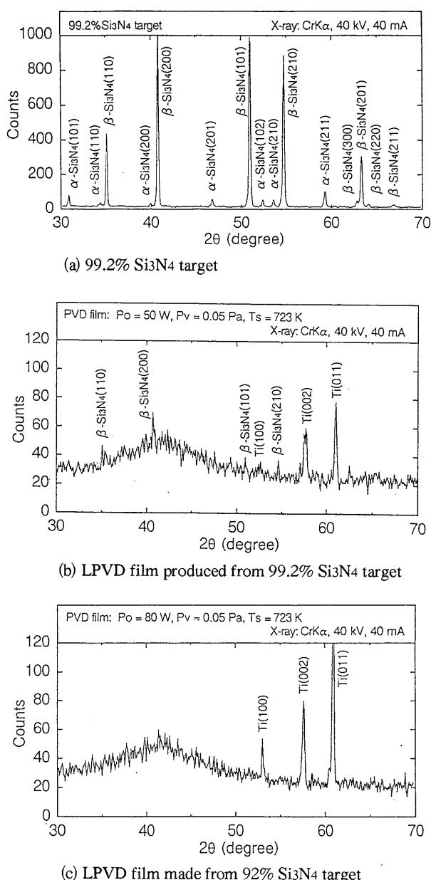
**Fig. 7** X-ray diffractometer result of  $\text{Si}_3\text{N}_4$  target and LPVD films produced on Ti substrate.
