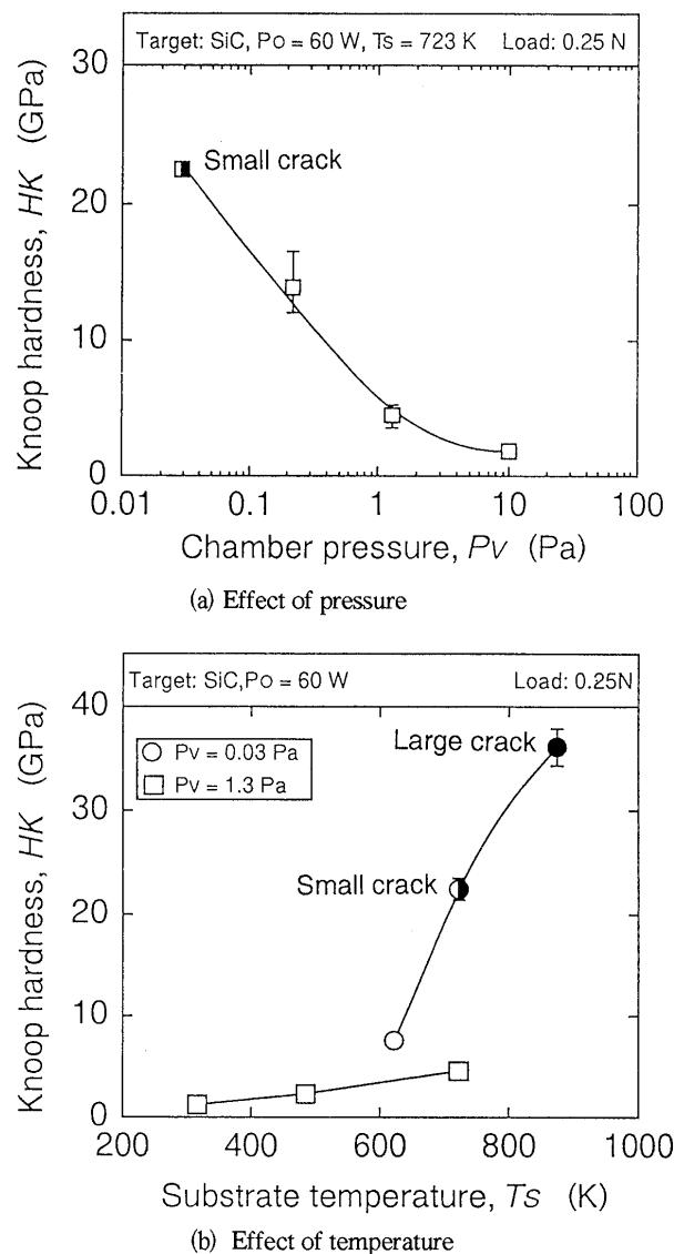
**Fig. 8** Effects of chamber pressure and substrate temperature on Knoop hardness of LPVD film surface produced from SiC target.
