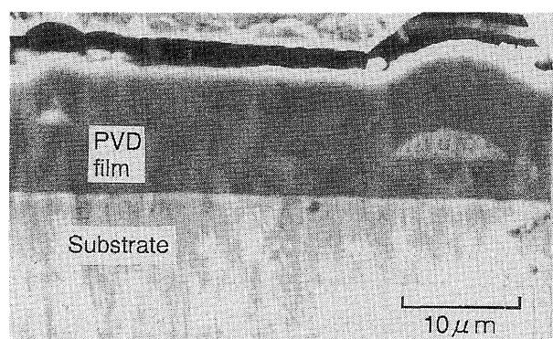
(b) 92.0%  $\text{Si}_3\text{N}_4$  target ( $P_o=80 \text{ W}$ ,  $P_v=0.06 \text{ Pa}$ )
