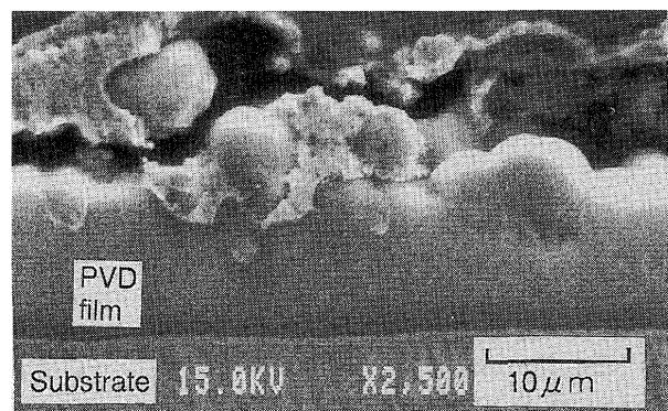
(a) 99.2%  $\text{Si}_3\text{N}_4$  target ( $P_o=50 \text{ W}$ ,  $P_v=0.03 \text{ Pa}$ )
