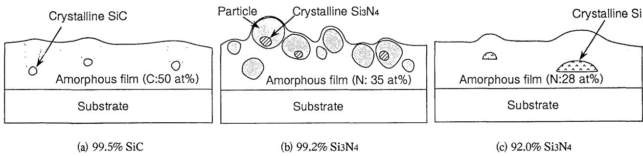
**Fig. 15** Cross-sectional schematic of LPVD films produced from SiC and Si<sub>3</sub>N<sub>4</sub> targets.
