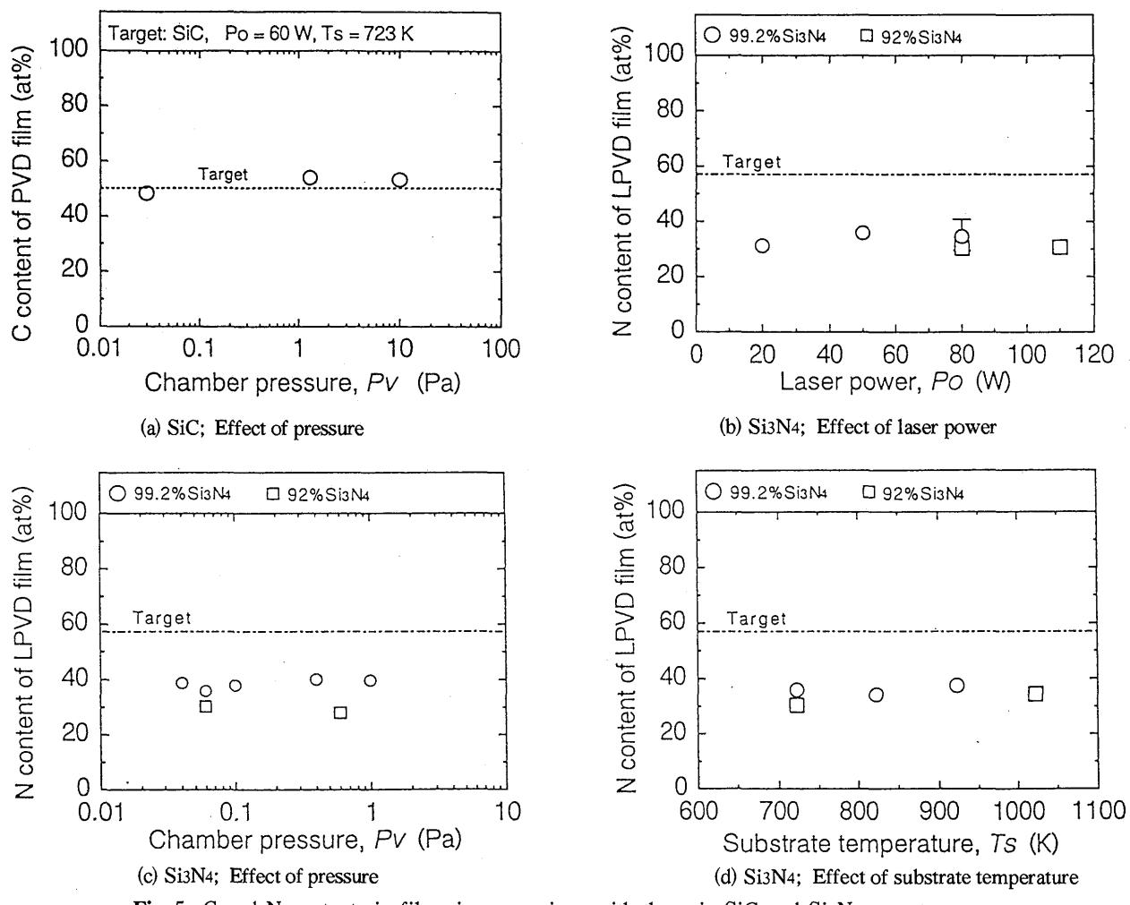
Fig. 5 C and N contents in films in comparison with those in SiC and Si<sub>3</sub>N<sub>4</sub> targets.
