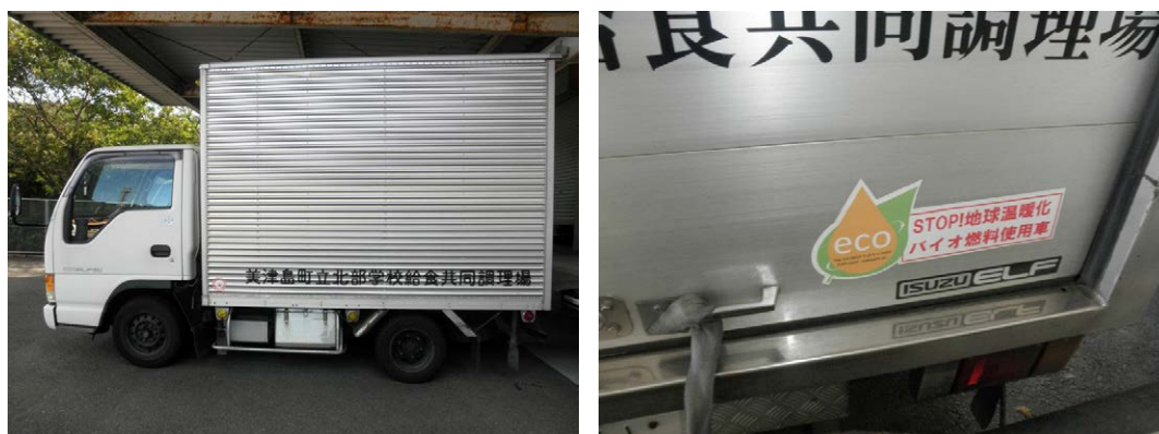
FIGURE 4. School lunch distribution truck using diesel fuel made from waste cooking oil. (Photo by the first author in 2011)
