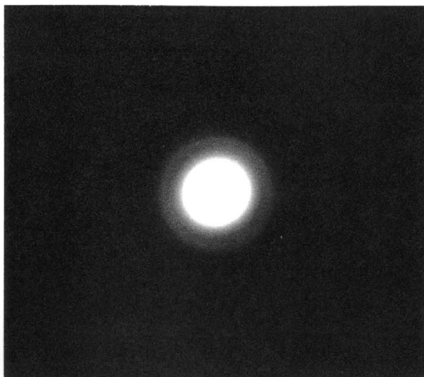
Figure 3.3. Electron diffraction pattern of the as-prepared CeO 2 -ZrO 2 ultrafine particles (Ce:Zr = 2:8).
