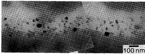
Fig.14 Electron micrographs of joint interfaces of 4N the pure Al bonded with the Al - 0.6% Mg intermediate layer ( t_w=3.6 ks, T_w=873 K, P_w=0.5 MPa).
