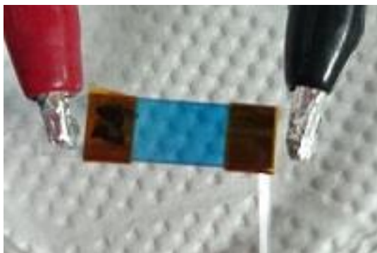
Figure 4-16 Photographs of PB-film electrolysis cell (a) before electrolysis and (b) about 20 min after applying V_{DC} = +3.0 V
