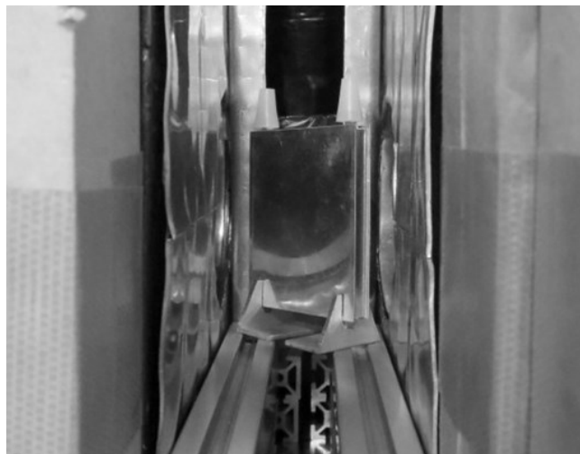
Fig. 2-13 Picture of the sample liquid holder used in the experiment.
