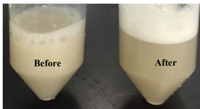
Figure 14: Suspended cell pellet before sonication (Before) and after the sonication completed (After).
