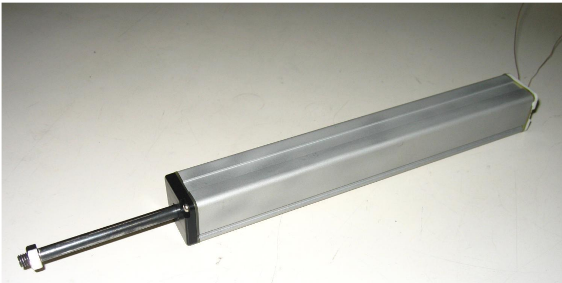
Fig.4.3 Prototype of contactless magnetic type position sensor
