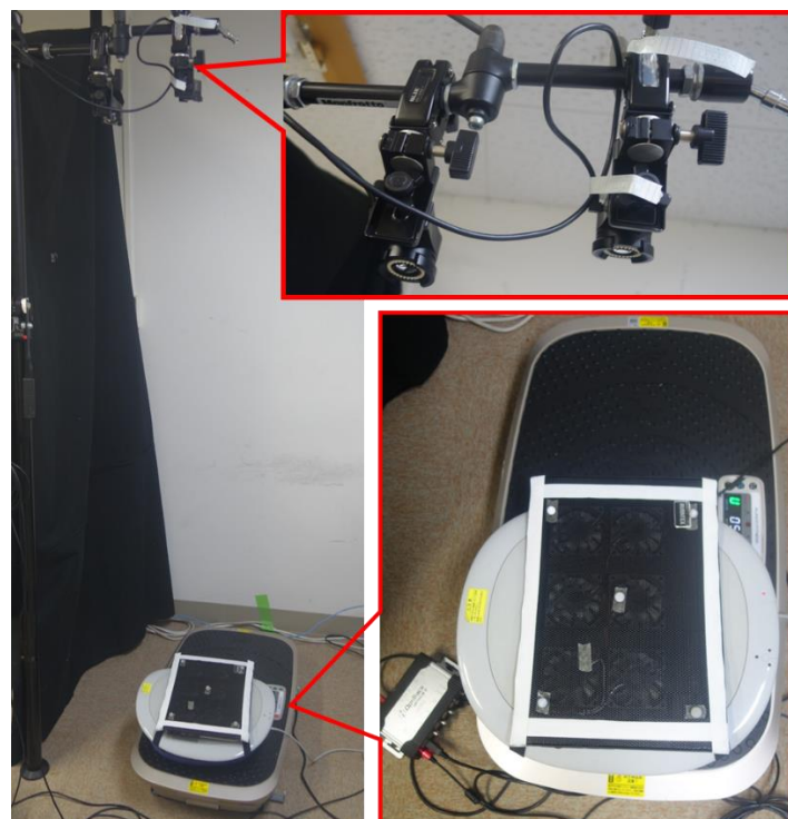
Figure 4.6 Using the OptiTrack to track the five markers attached on the panel, we examined the shaking movements of the panel to ensure that the simulations of essential tremor and intentional tremor were accurate.
