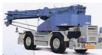
(f) Rough terrain crane
