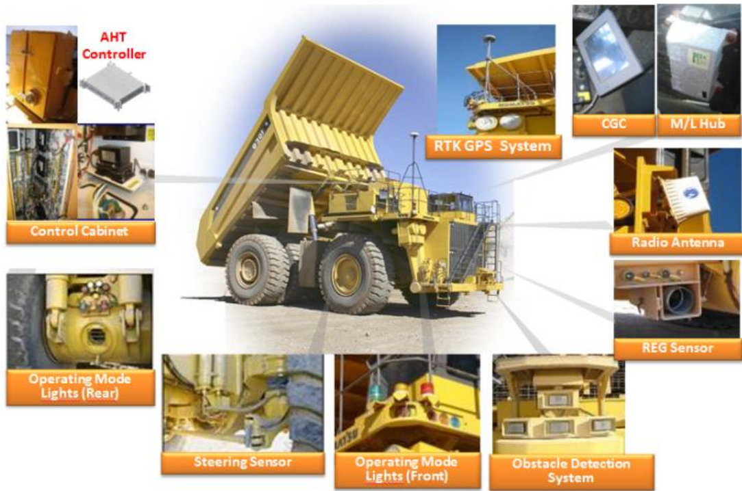
Fig.2-10 New technologies for driverless trucks.
