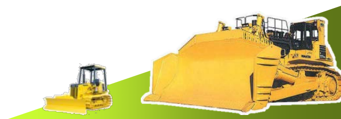
(b) Bulldozer. Machine weight : 3,940kg – 152,600kg, 39 times
