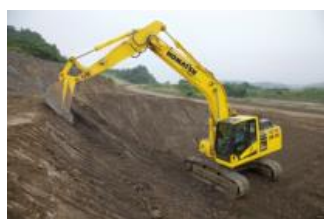
(a) Hydraulic excavator
