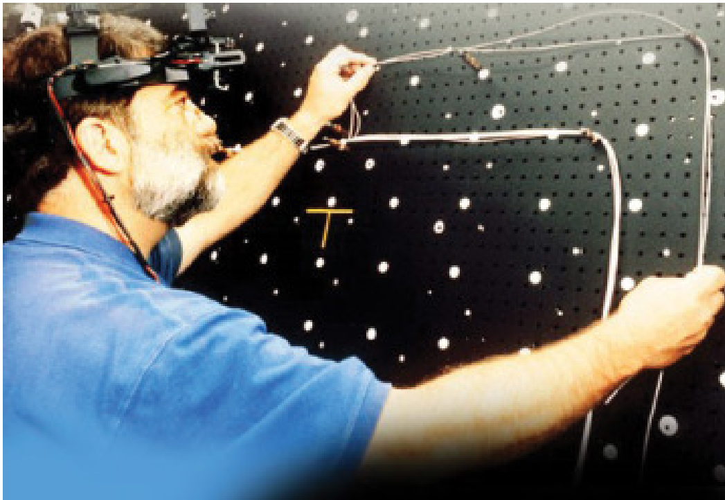
Figure 2.17: A small head-mounted video camera to display a diagram and text on the workpiece [11] .
