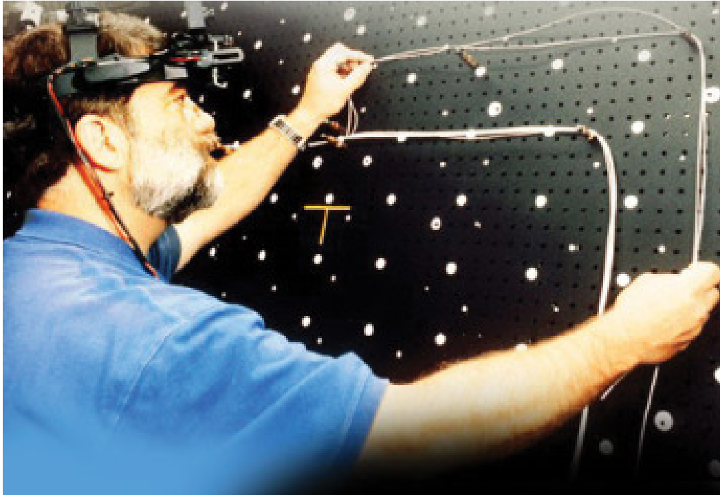
Figure 2.17: A small head-mounted video camera to display a diagram and text on the workpiece [11] .
