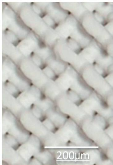
**Fig.** An alumina micro lattice with a diamond type periodic pattern fabricated by using ultraviolet stereo-lithography. The ceramic component was formed from resin paste including nanoparticles through dewaxed and sintered by ultraviolet laser beam scanning.
