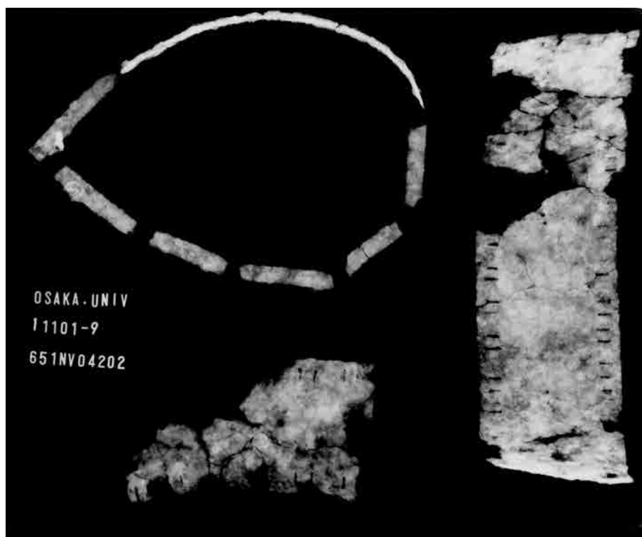
Fig. 8 X-ray radiography of iron bordering and neck plate no. 8
