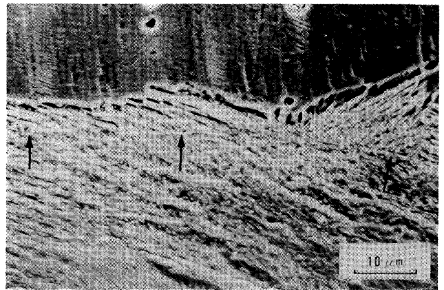
Fig. 12 An example of prior \gamma grain-boundary observed in carbide layer, indicated by arrows
