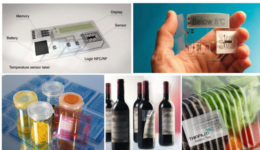
Figure 1.7 All-printed smart temperature sensor tag for medicine and food traceability management [3, 4].
