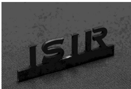
Figure 5.3 One sample of electrical discharge machining of Al_2O_3/20\% Ti composite.
