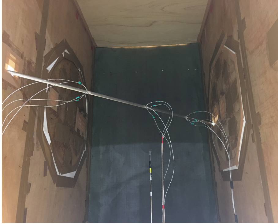
Fig. 4.15: Conductor placement in wind tunnel outlet
