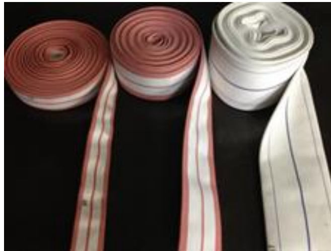
Fig. 3.5 Fire-hoses having different diameters used in bending stiffness measurements (40mm, 65mm and 100mm diameter)
