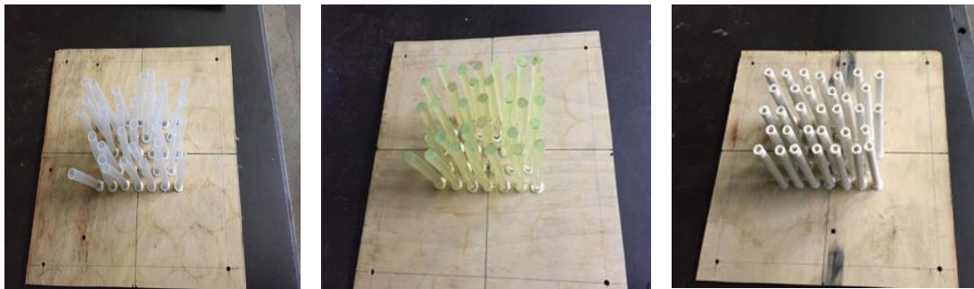
Fig. 4.11 Silicone rubber pipe, urethane rubber pipe and rigid ABS pipes
