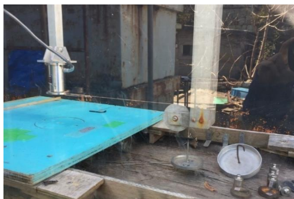
Fig. 4.7a Force transducer calibration arrangement
