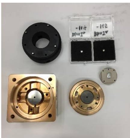
Fig. 2-9 The DAC used for synchrotron powder XRD.
