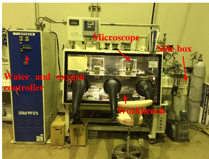
Fig. 2-23 the glovebox for loading sample in insert atmosphere.
