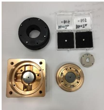
Fig. 2-9 The DAC used for synchrotron powder XRD.
