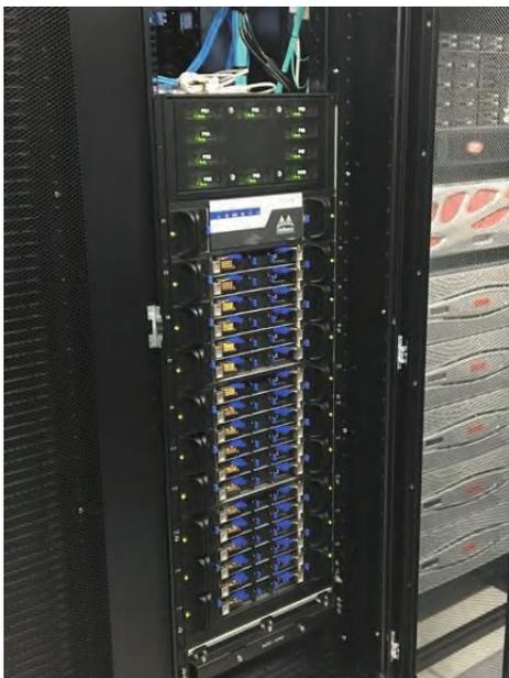
図 18 CS7500 InfiniBand Director Switch
