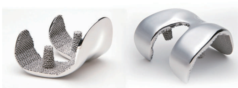
Fig. 2 EBM-built artificial knee joints after polishing.
