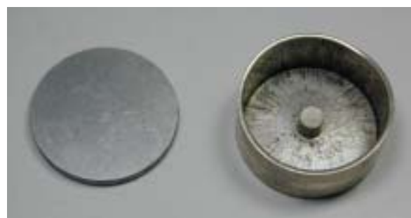
(a) Initial ZK60 billet (b) Forged ZK60 billet ( D_0 = 30\text{mm} , H_0 = 3.0\text{mm} )
