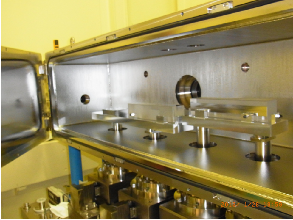
Figure 4.6: The Kirkpatrick-Baez mirror at BL19LXU in SPring-8
