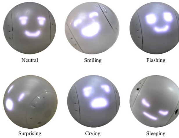
Figure 5.4: LED patterns implemented for the eyes and mouth of the robot.
